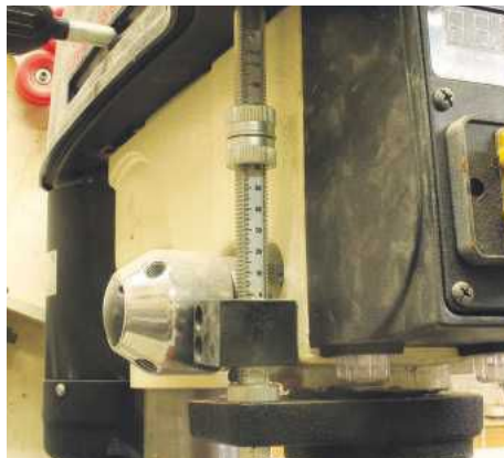
▲ Pic.11 He has set the stop on his drill press to give him the exact depth for the tea light. Its diameter is 38mm so he has a saw-tooth machine bit the exact size
